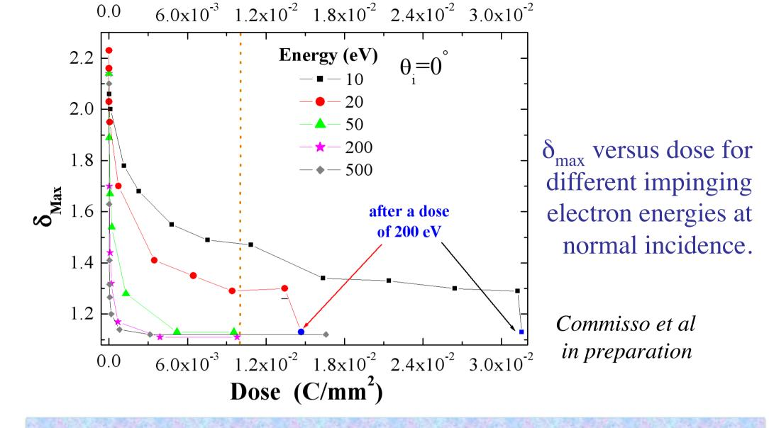
We demonstrate that the potentiality of an electron beam to reduce the SEY does not only depend on its dose, but also on hits energy.
