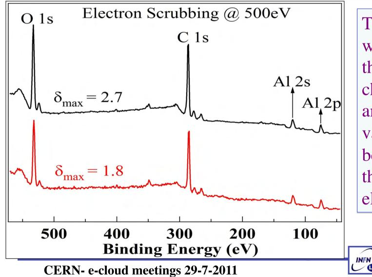
The XPS spectra were acquired on the Al sample characterized bv an initial  $\delta \max$ value of 2.7 eV, before and after the exposure to the electron dose.
