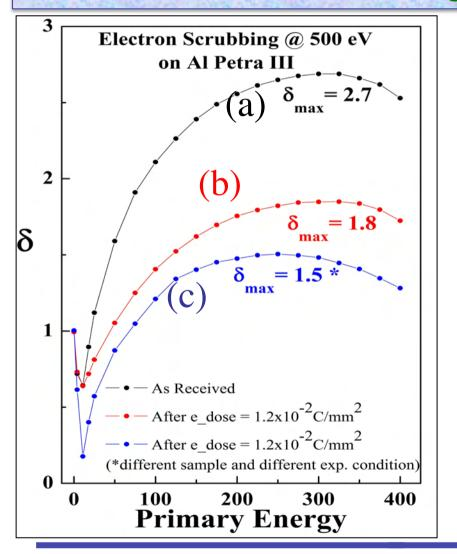
Three SEY spectra recorded in different conditions on Al technical samples cut from the inner walls of the Petra III storage ring, (a) "as received" (b) after electron scrubbing at 500 eV KE in UHV at background pressures of low 10<sup>-9</sup> (c) after electron scrubbing at 500 eV KE in UHV at background pressures of low 10<sup>-10</sup> mbar
